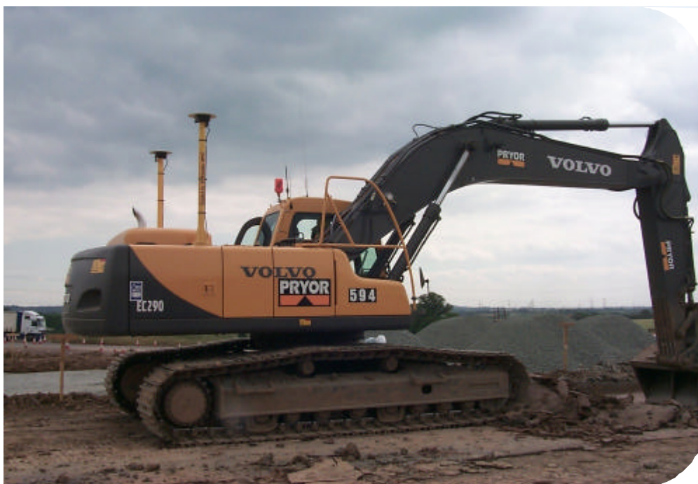
PCX 3D in action ... highway construction in boulder clay
