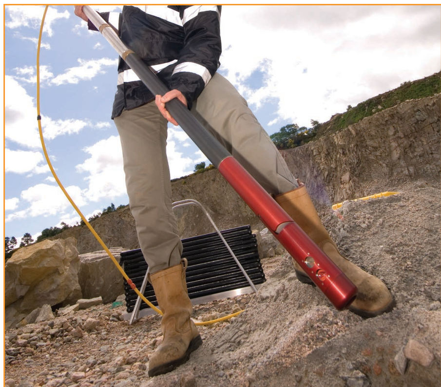
The probe rotates on two axes to create full 360-degree scans of voids and cavities.
