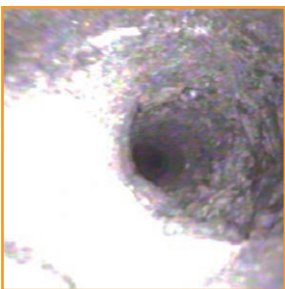
The nosecone camera provides a helpful view into the borehole during deployment.
